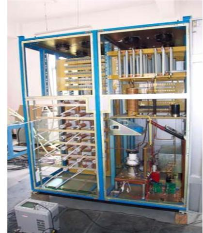
Figure 2. The PFN and switch cabinet
